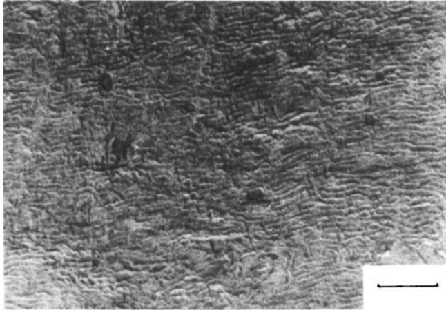
FIGURE 7 TEM replica of the etched-surface of the recrystallized sample. Note that the lamellar overgrowth masks entirely the shish structure (bar length = 0.5  $\mu\text{m}$ ).
