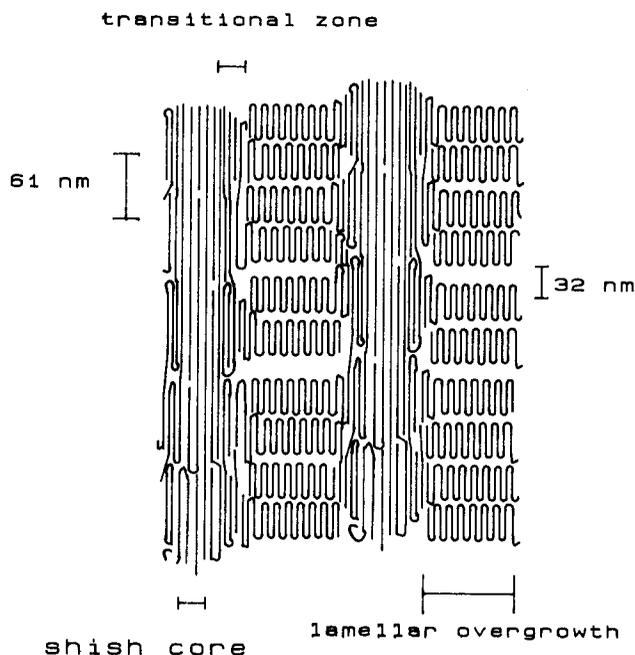
FIGURE 2 Sketch of the proposed shish-kebab structure including the shish core, the transitional zone and the overgrown lamella (kebabs).
