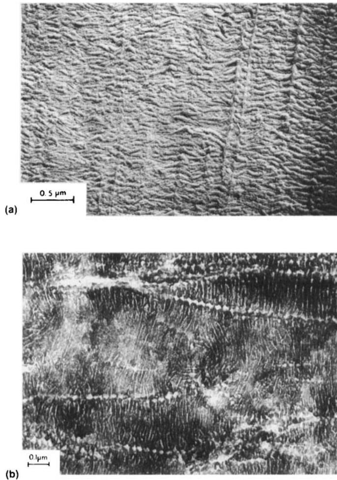
FIGURE 1 Transmission electron-micrographs of the investigated sample: (a) etched-surface replica, (b) ultrathin stained section.
