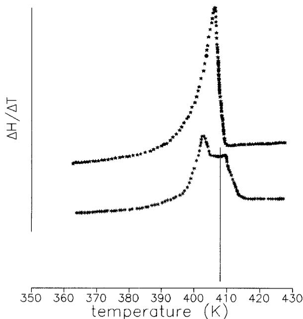
FIGURE 5 DSC traces showing the two melting maxima corresponding to the original sample (lower trace). The lower peak is associated to the melting of the overgrown lamellae while the higher one corresponds to the melting of the shishes. The upper trace corresponds to the melting of the recrystallized structure (see the electron-micrograph in Figure 7). Vertical line indicates the maximum annealing temperature during the SAXS experiments.
