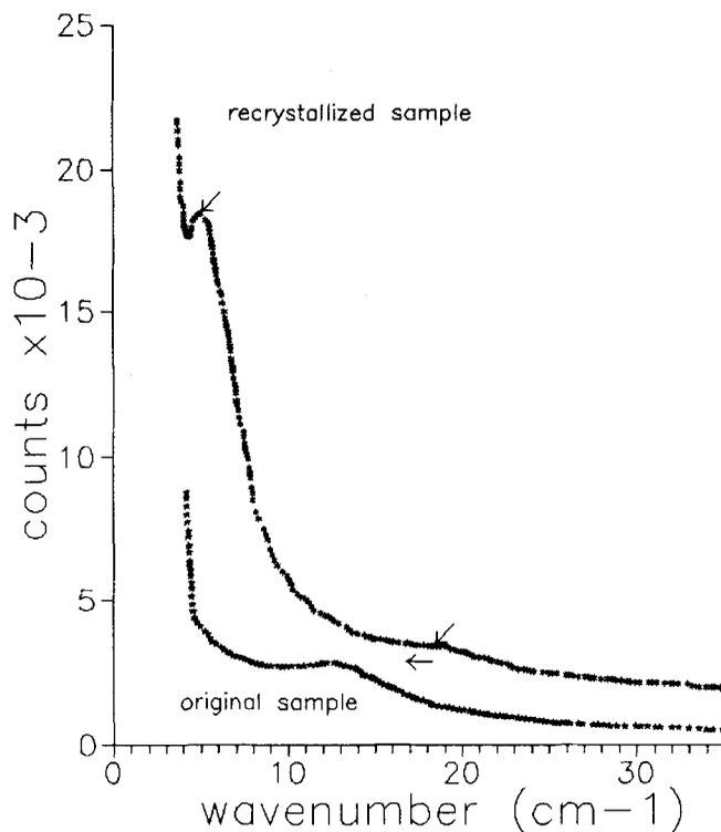
FIGURE 6 Raman spectra of the original and recrystallized samples. LAM modes of each sample are indicated by arrows.
